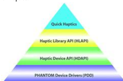
Figure 3: Layers of the QuickHaptics
