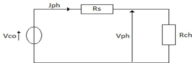
Figure 6: Equivalent circuit of the photocell (real voltage generator)
