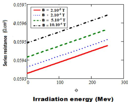
Figure 7: Variation of the series resistance according to the irradiation energy for different values of the magnetic field
