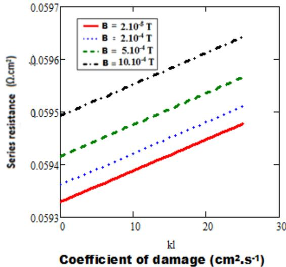
Figure 8: Variation of the series resistance according to the coefficient of damage for different values of the magnetic field
