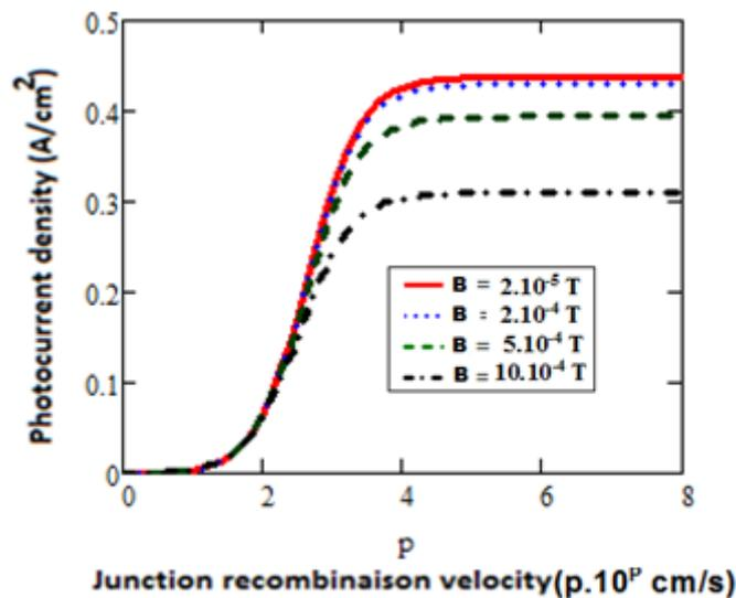
Figure 3: Variation of the photocurrent density versus recombination velocity at the junction for different values of the applied magnetic field
