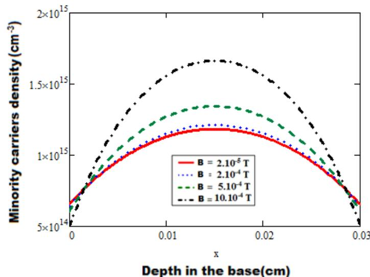
Figure 2: Variation of the minority charge carriers according to the thickness of the base for different values of the magnetic field
