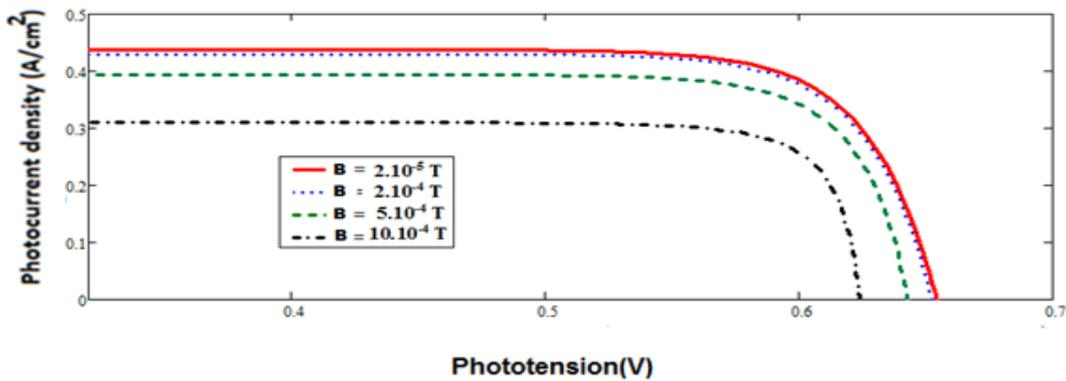
Figure 5: I-V characteristic of the solar cell
