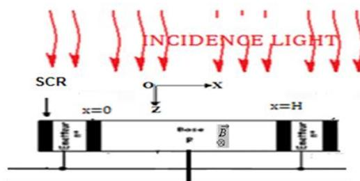
Figure 1: Parallel vertical junctions of a solar cell
