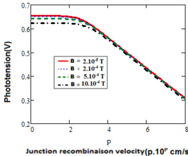
Figure 4: Variation of the phototension according to the recombination velocity at the junction for different values of the applied magnetic field
