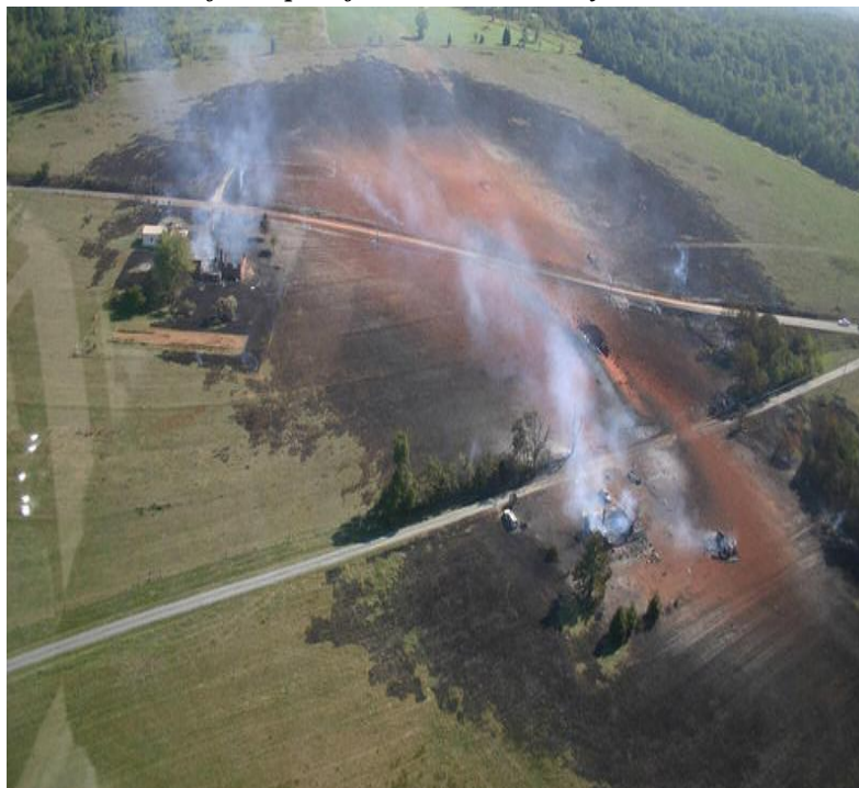
Figure 6: A view of the damage caused due to failure of a Gas pipeline. The Failure was caused due to 3rd Party activity [Source: NTSB, USA]
