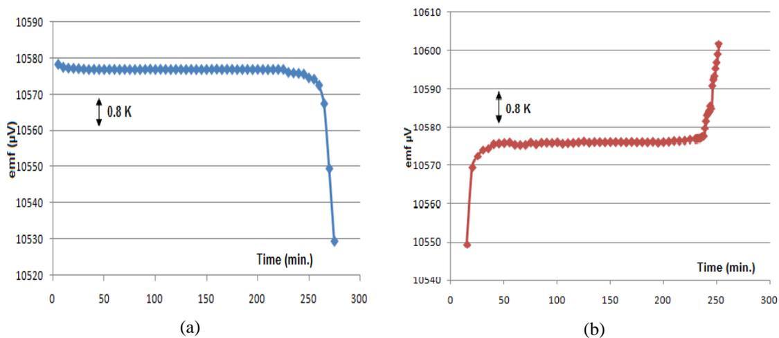
Figure 1: Melting and Freezing plateaus of the Copper cell using type S thermocouple
