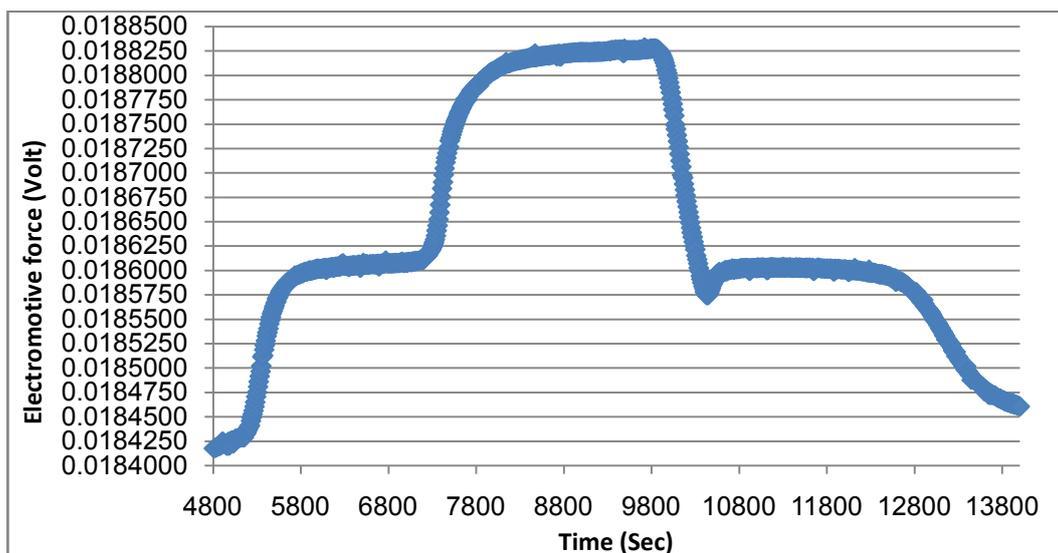
**Figure 2:** Melting and freezing points of Pt/Pd thermocouple in Co-C eutectic fixed point
