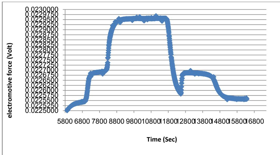
Figure 3: Melting and freezing points of Pt/Pd thermocouple in Pd-C eutectic point
