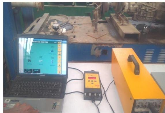
*Figure 4: Emission measurement system overview*
