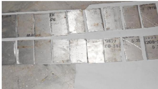
Figure 2: Test specimens of aluminium alloy AA6061
