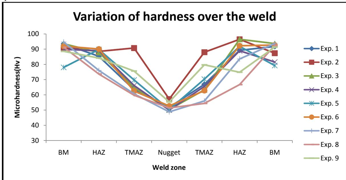
Figure 8: Microhardness of all as welded specimens
