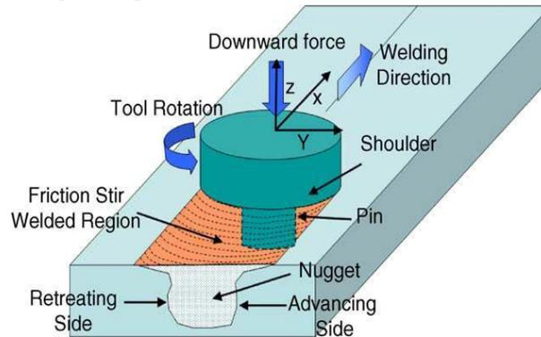
Figure 1: Schematic diagram of friction stir welding [5]
