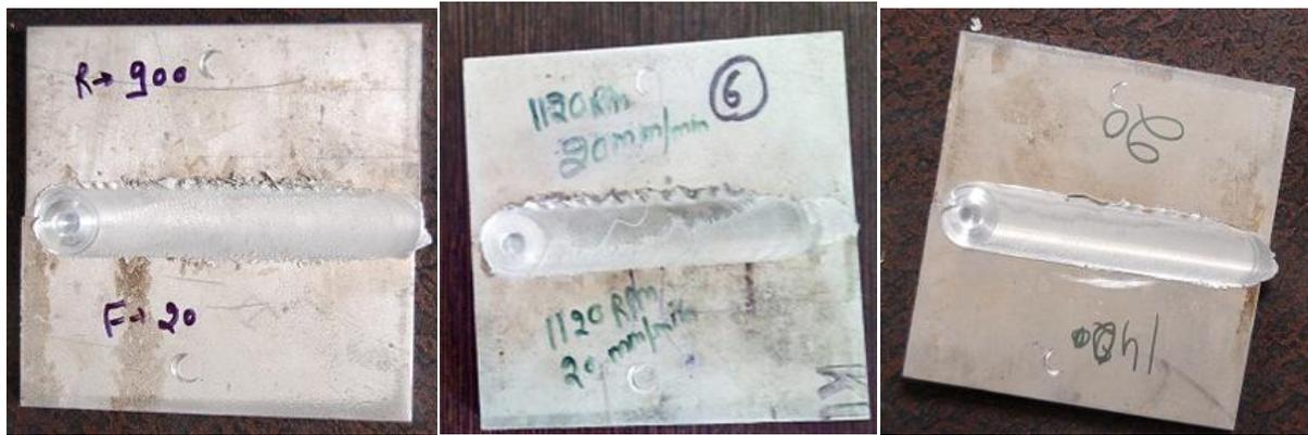
Figure 5: Friction stir welded AA6061-T651 alloy specimens
