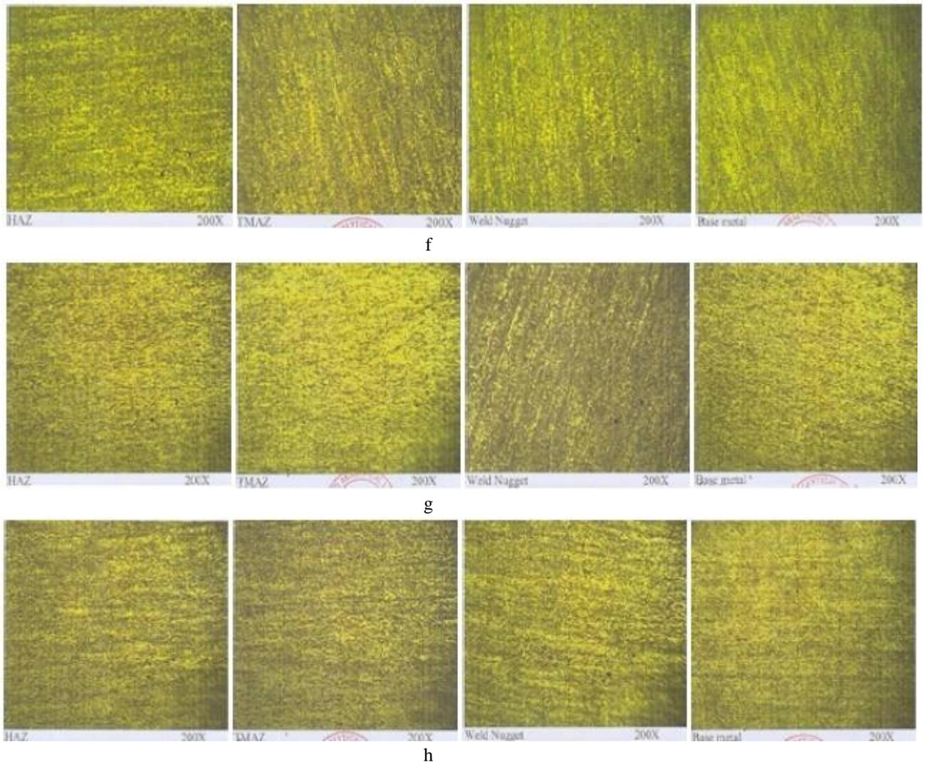
Figure 7: Microstructure of (a) specimen 1 (900 rpm and 20 mm/min) (b) specimen 2 (900 rpm and 25 mm/min) (c) specimen 3 (900 rpm and 30 mm/min) (d) specimen 4 (1120 rpm and 20 mm/min) (e) specimen 5 (1120 rpm and 25 mm/min) (f) specimen 6 (1120 rpm and 30 mm/min) (g) specimen 7 (1400 rpm and 20 mm/min) (h) specimen 8 (1400 rpm and 25 mm/min) (i) specimen 8 (1400 rpm and 30 mm/min)
