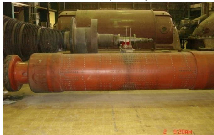
Figure 11: Alternator with the location (empty in the form of small white holes on the side surface of the alternator) of balancing balances
