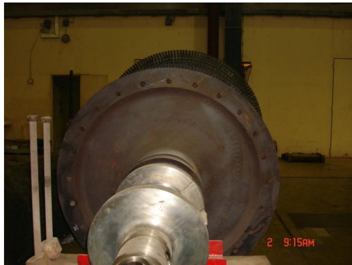
Figures 10: Low pressure 301 turbine with the location (empty in the form of white holes on the circumference of the turbine section) of balancing balances
