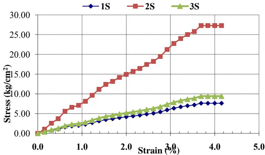
Figure 5: Unconfined compressive strength for samples S1, S2 and S3
