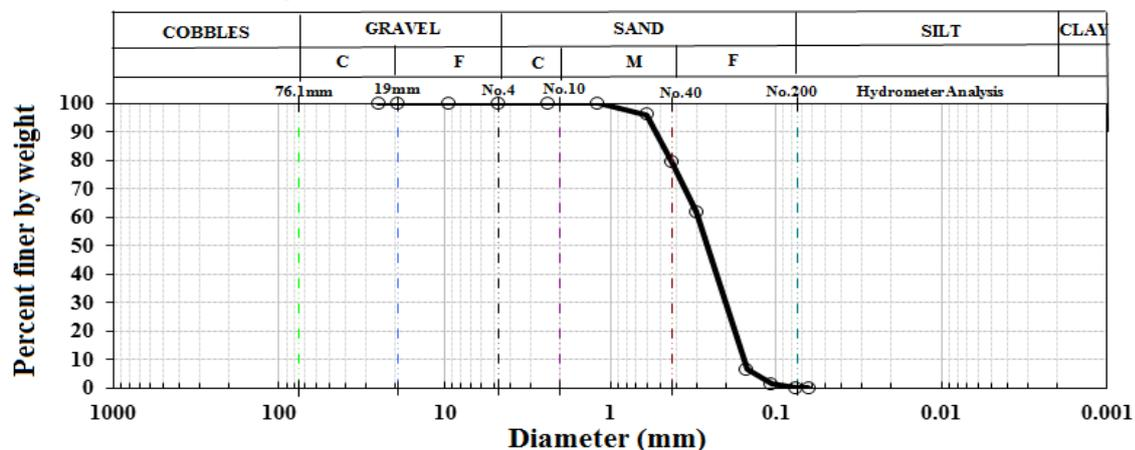
Figure 1: Grain size distribution curve of the natural tested siliceous sand
