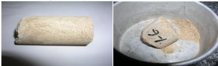
Figure 4: S3 before and after immersion with water
