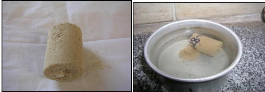
Figure 2: S1 before and after immersion with water
