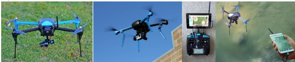
Figure 1: Images of IRIS + which can be used with gimbals, cameras and other sensors
