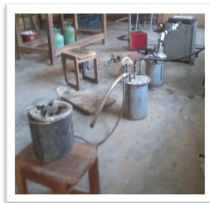
Figure 1: Complete Pyrolysis Experimental Setup
