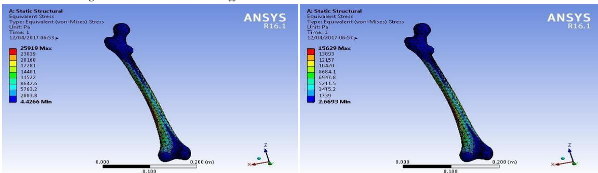
Figure 1.2: The maximum and minimum von mises stress on the bone without crack
