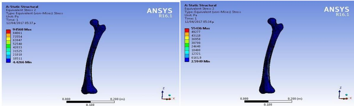
Figure 1.1: The maximum difference in von mises stress on the bone without crack
