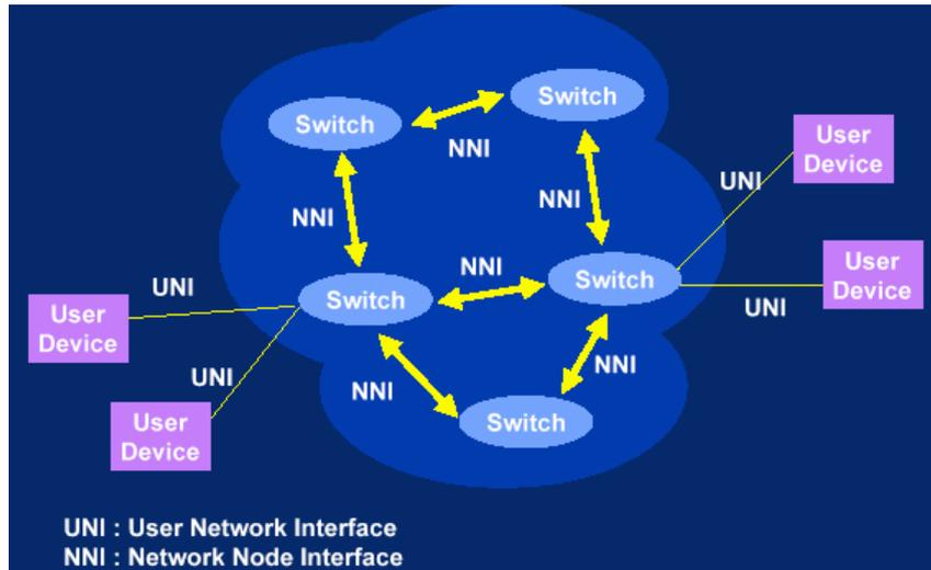
Figure 1: ATM Network using UNI and NNI Interfaces
