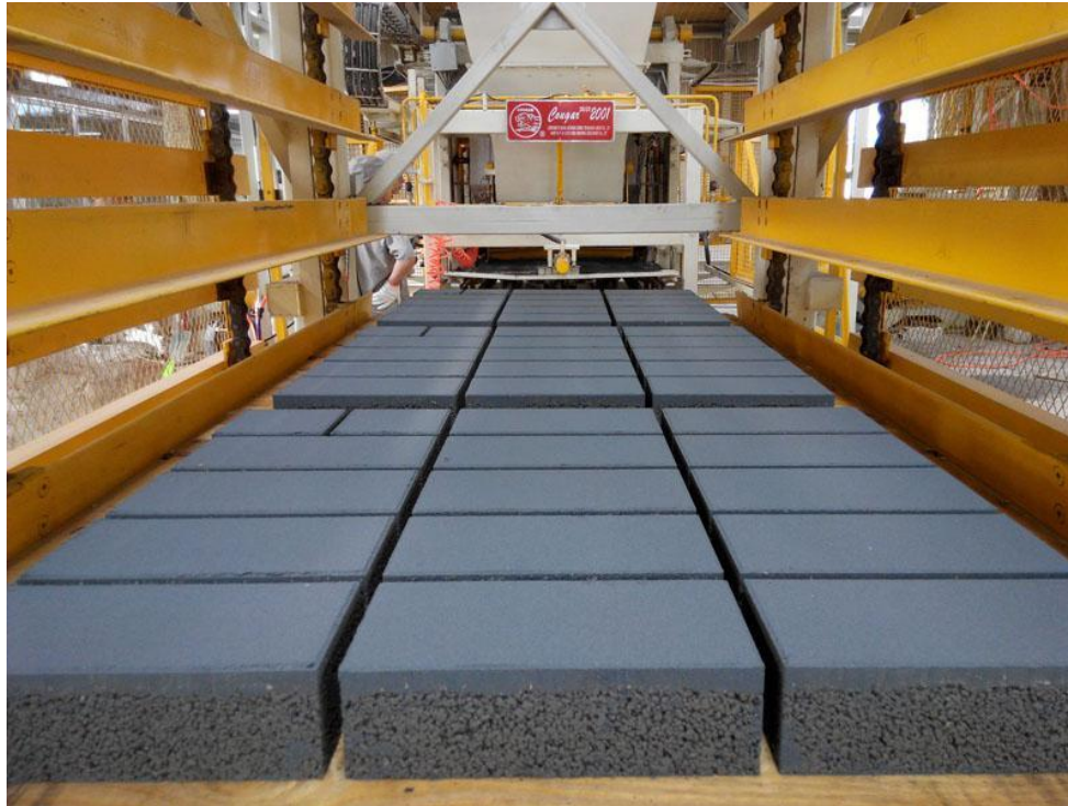
Figure 4: Prefabricated water permeable brick
