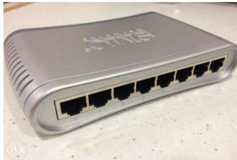
Figure 6: SMCFS8 Ethernet Switch
