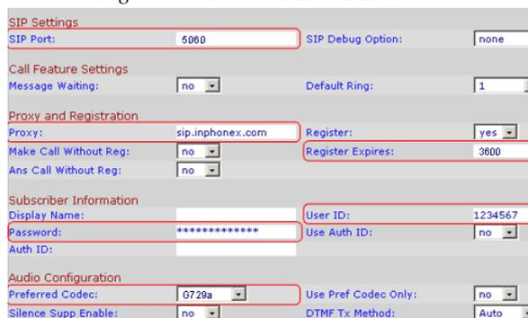
Figure 5: Cisco SPA 942 Configuration interface
