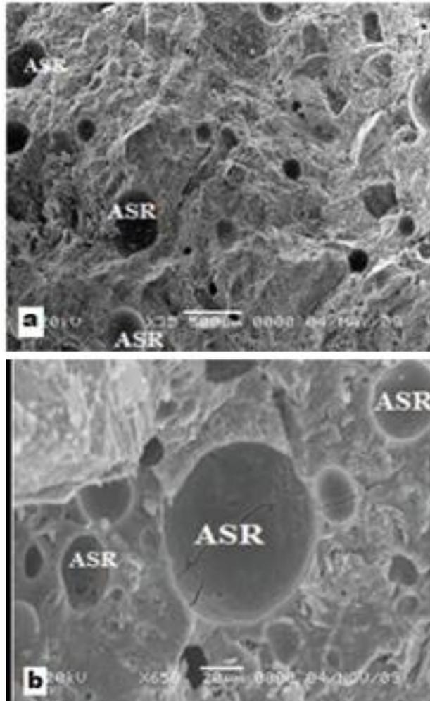
Figure 3: ASR products monitored via SEM
