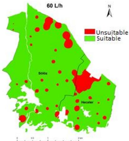
Figure 3.7: Suitable areas for mini sprinkler irrigation method (60L/h)
