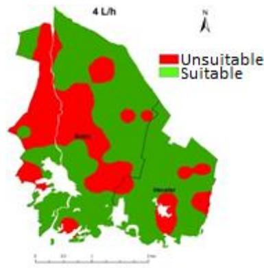
Figure 3.4: Suitable areas for drip irrigation method (4L/h)
