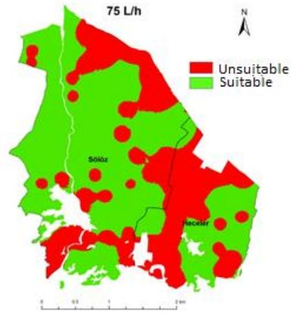
Figure 3.8: Suitable areas for mini sprinkler irrigation method (75L/h)
