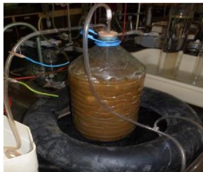
Figure 3: Digester with cow dung and water mixture
