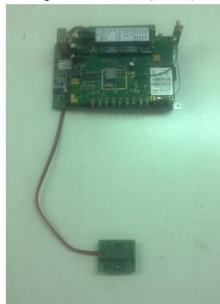
Figure 4: Energy meter at nodes B and C plus radio unit
