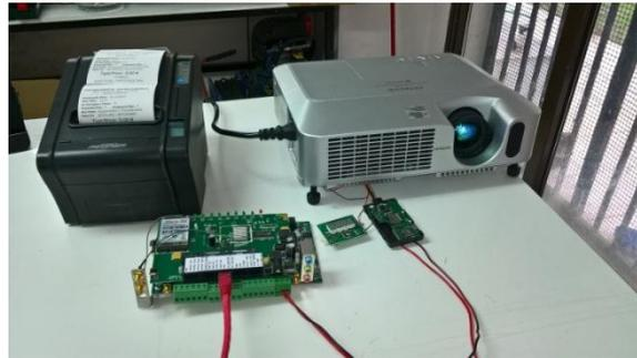
Figure 7: Set up for Node C (projector and thermal printer)
