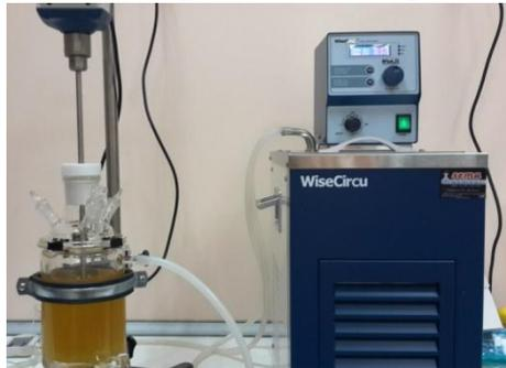
*Figure 2: Laboratory scale biodiesel reactor*
