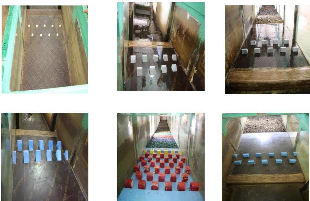
*Figure 3: Geometry of Stilling Basin and Baffle Blocks*
