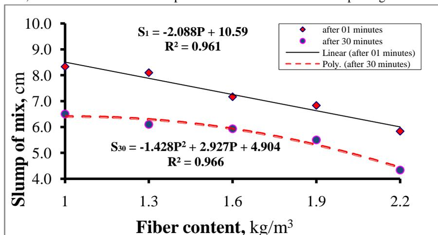
**Figure 2:** Relationship between fiber content and slump
