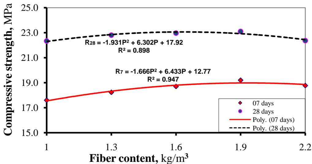
Figure 3: Relationships between fiber content and compressive strength
