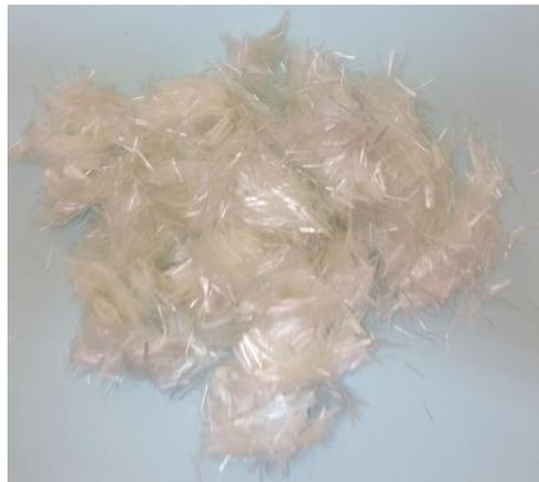
Figure 1: Polypropylene fiber
