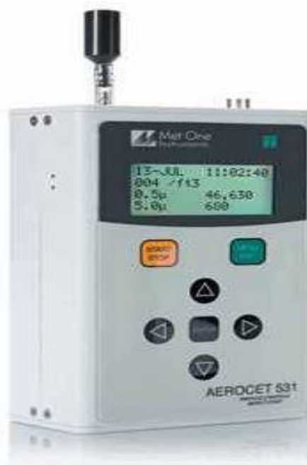
Figure 1: Mass Particle Counter (Aerocet-531S) used for investigation of Particulate Matter
