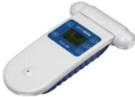
Figure 2: Gas monitor (Aeroqual series 500) used for investigation of all the gaseous pollutants monitored
