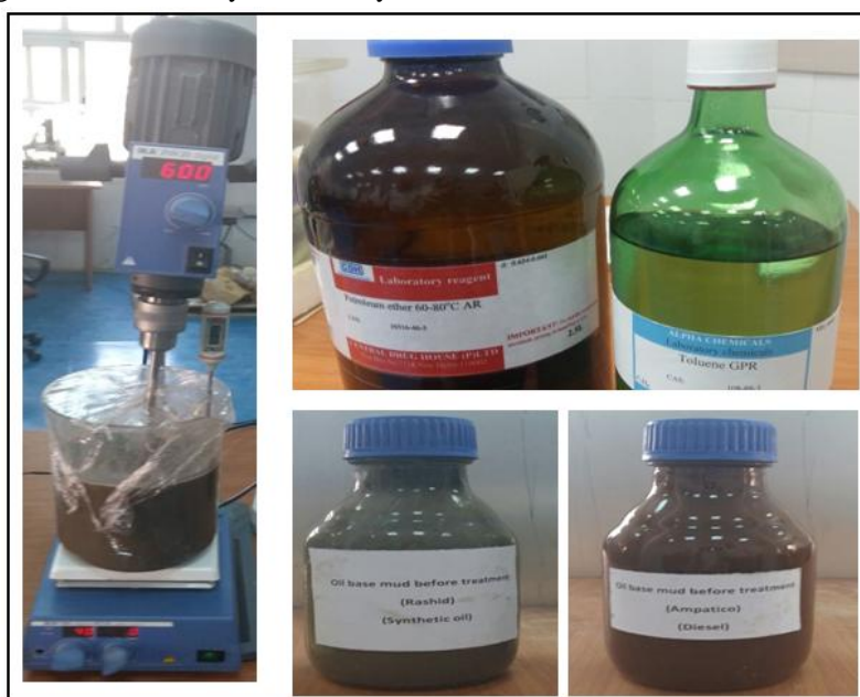
Figure 1: Photographs of a stirring system, solvents and contaminated cuttings
