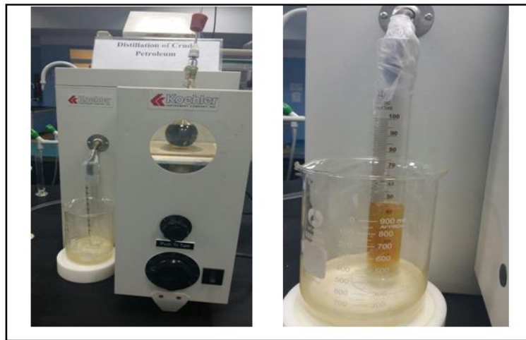
Figure 2: Photographs of ASTM distillation unit with receiving products
