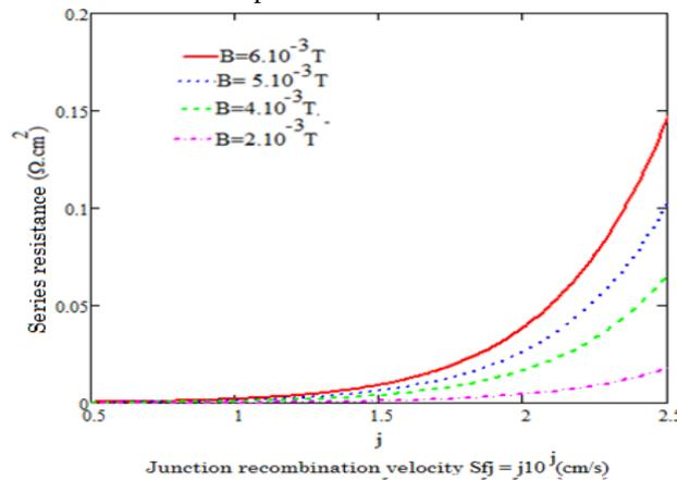
Figure 5: Series resistance versus junction recombination velocity for different values of the magnetic field.
