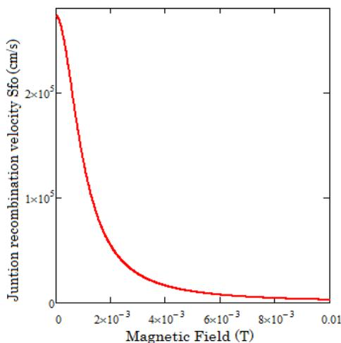
Figure 1a : Junction recombination velocity  $Sfo^*$  versus magnetic field
