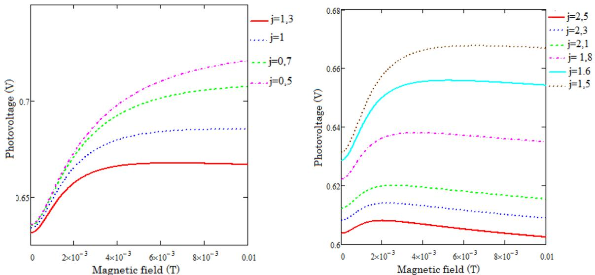
Figure 2: Photovoltage versus magnetic field for different values of the junction recombination velocity near the open circuit
