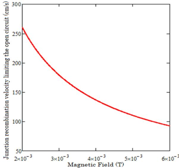
Figure 4: The junction surface recombination velocity of minority charge carriers limiting the open circuit versus of magnetic field
