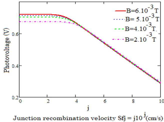
Figure 3: Photovoltage versus junction recombination velocity for different values of the magnetic field. ( $D=26\text{cm}^2/\text{s}$ ,  $\mu=10^3\text{cm}^2.\text{V}^{-1}\text{s}^{-1}$ ,  $\tau=10^{-5}\text{s}$ ,  $H=0,03\text{cm}$ )
