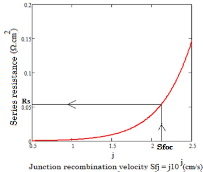
Figure 6: Determination of the series resistance
