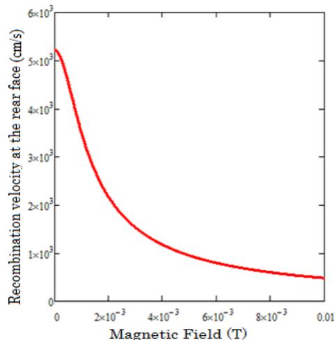
Figure 1b : Recombination velocity at the rear face  $Sb^*$  versus magnetic field
