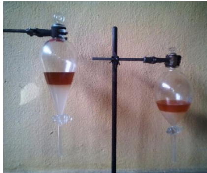
Figure 3: Separation of biodiesel (Top layer) and water (bottom) layer after washing and glycerol (bottom) layer
