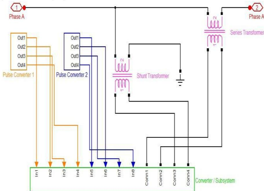
Figure 5: Unified Power Flow Diagram
