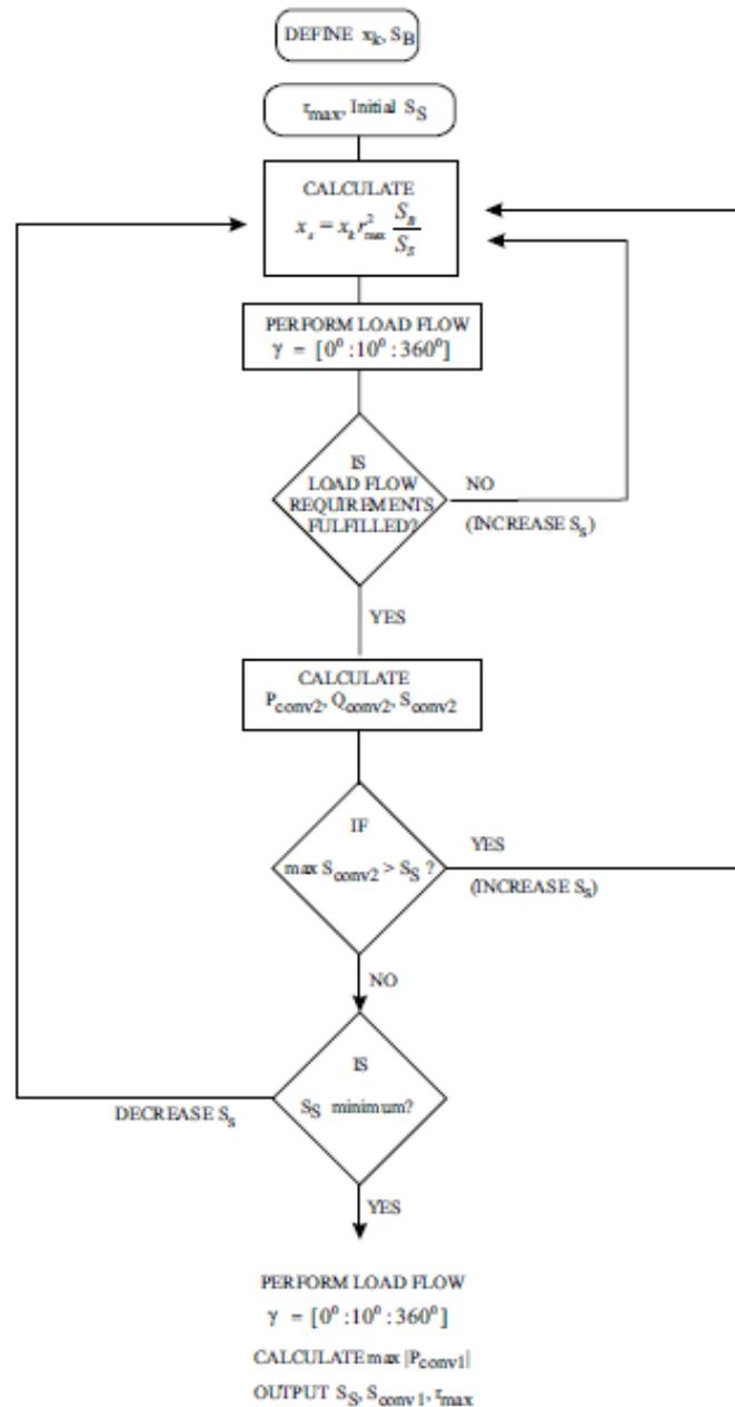
Figure 1: Algorithm for optimal rating of the UPFC
