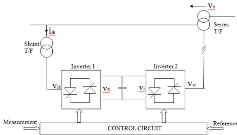
Figure 2: UPFC installed in transmission line
