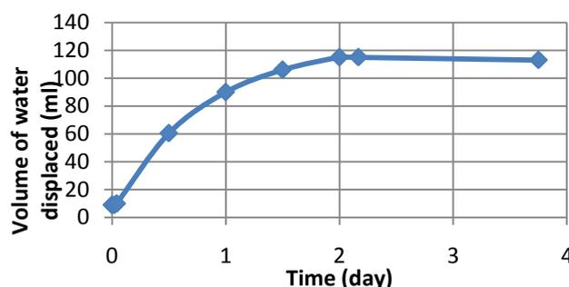
*Figure 8: Graph of volume of water displaced (ml) per unit time (day)*
