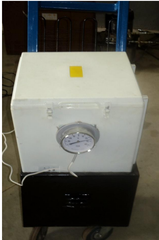
The experimental refrigerator
