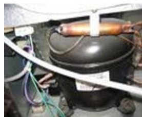
The hermetic Compressor Source[5].
