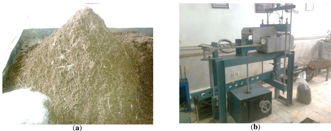
Figure 2: (a) Soil and fiber mixing; (b) Large scale (30cm*30cm) direct shear test device.
