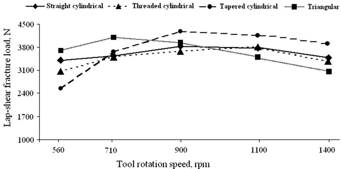
Figure 6: The effect of the tool pin profile on weld strength of PP welds.
