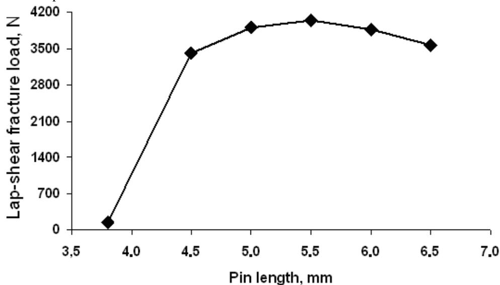
Figure 10: The effect of the pin length on the lap-shear fracture load of PP welds.
