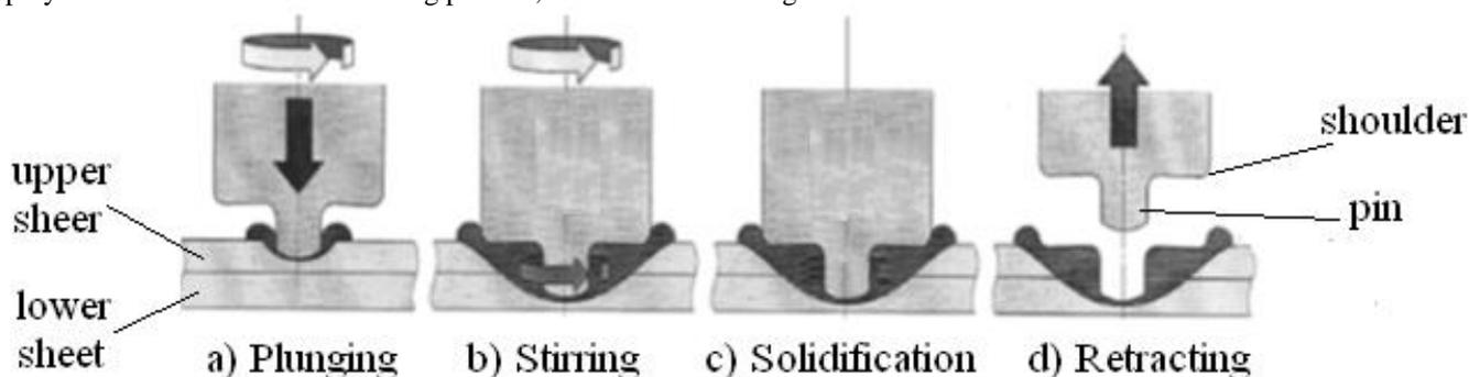
Figure 1: Four phases of friction stir spot welding process: (a) plunging, (b) stirring, (c) solidifying and (d) retracting [3].
