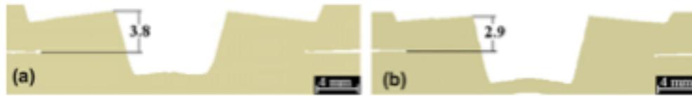
Figure 12: The effect of pin length on the thickness of the upper sheet of HDPE welds (a) 5.5 mm pin length and (b) 6.5 mm pin length.
