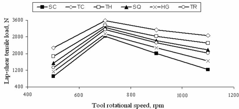
Figure 5: The effect of the tool pin profile on weld strength of HDPE welds.
