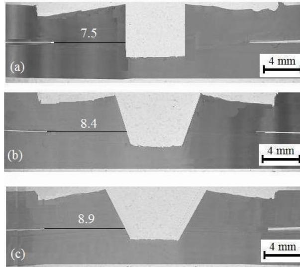
Figure 9: The effect of pin angle on weld stir zone formation of PP welds (a) threaded straight cylindrical pin, (b) 15° pin angled tapered cylindrical pin and (c) 25° pin angled tapered cylindrical pin.
