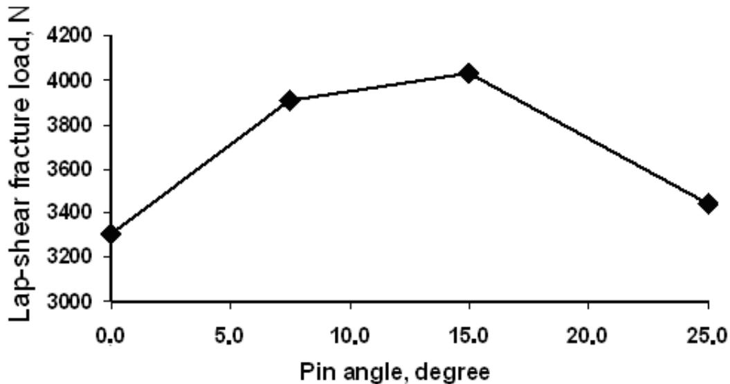
Figure 8: The effect of pin angle on the lap-shear fracture load of PP welds.
