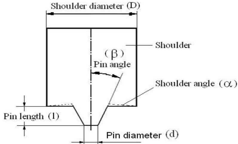
Figure 3: Friction stir spot welding tool design showing geometric parameters.
