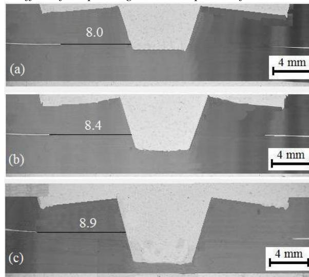
Figure 11: The effect of the pin length on the weld cross sections of PP welds (a) 4.5 mm pin length, (b) 5.5 mm pin length and (c) 6.5 mm pin length.
