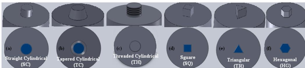
Figure 4: FSSW tool profile and pin size (a) straight cylindrical, (b) tapered cylindrical and (c) threaded cylindrical.
