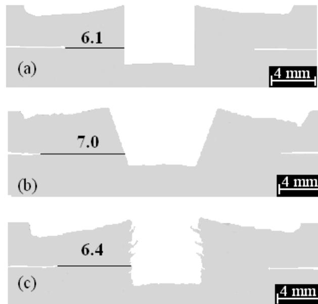
Figure 7: Effect of pin angle on weld nugget formation HDPE welds (a) straight cylindrical pin, (b) 15° pin angled tapered cylindrical pin and (c) threaded straight cylindrical pin.
