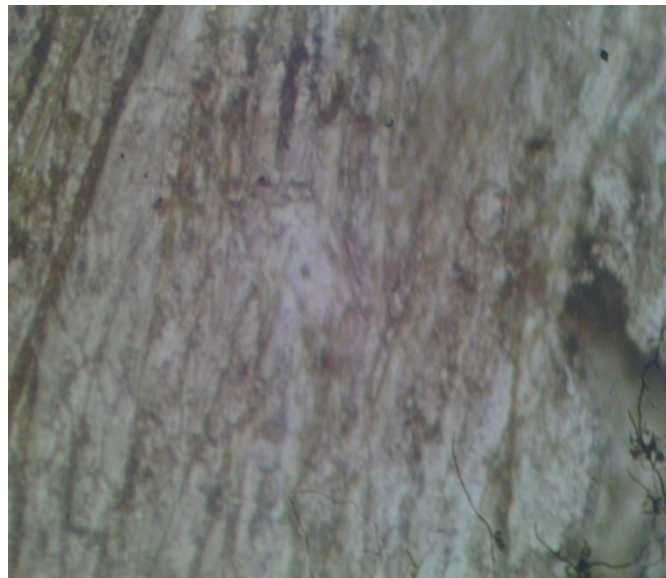
Plate 1: Micrograph of Al-12%Si alloy as-cast.
