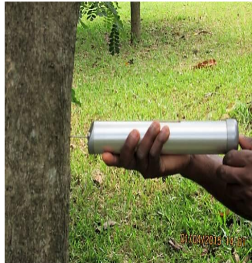
Figure 2: The pilodyn 6 joules (wood tester) used for experimentation.
