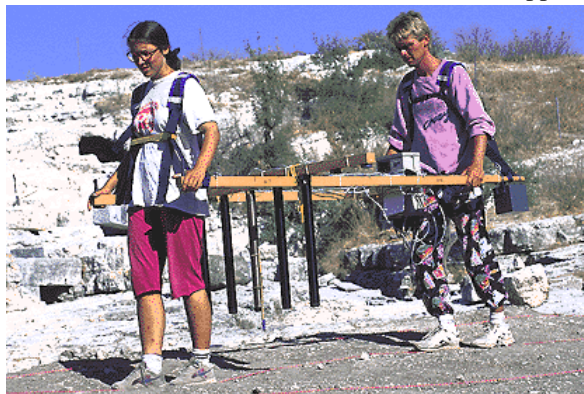
Figure 4: Kuşaklı-Sarissaregion using Flux-gatemagnetometers.
