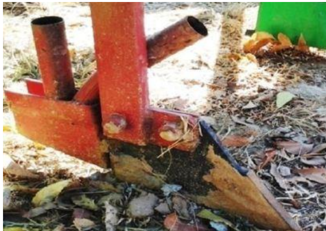
Figure 2: Shoe Type Furrow Opener
