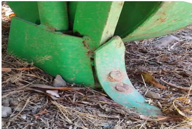
Figure 3: Shovel type furrow opener
