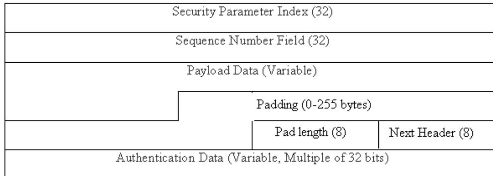
*Figure 2: IPsec ESP Header Format.*
