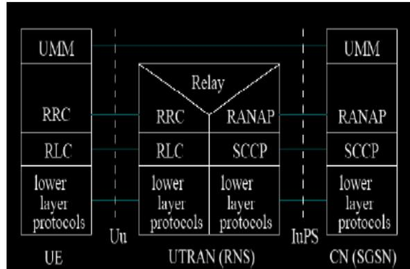
**Figure 1:** Control plane of UMTS mobility management between UE – UTRAN and cn – CN [14]
