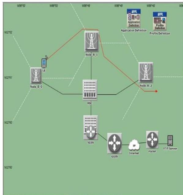
Figure 4: Network diagram by using OPNET
