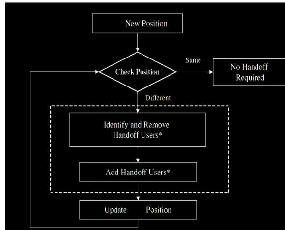
**Figure 2:** Immediate Handoff Initiation Algorithm
